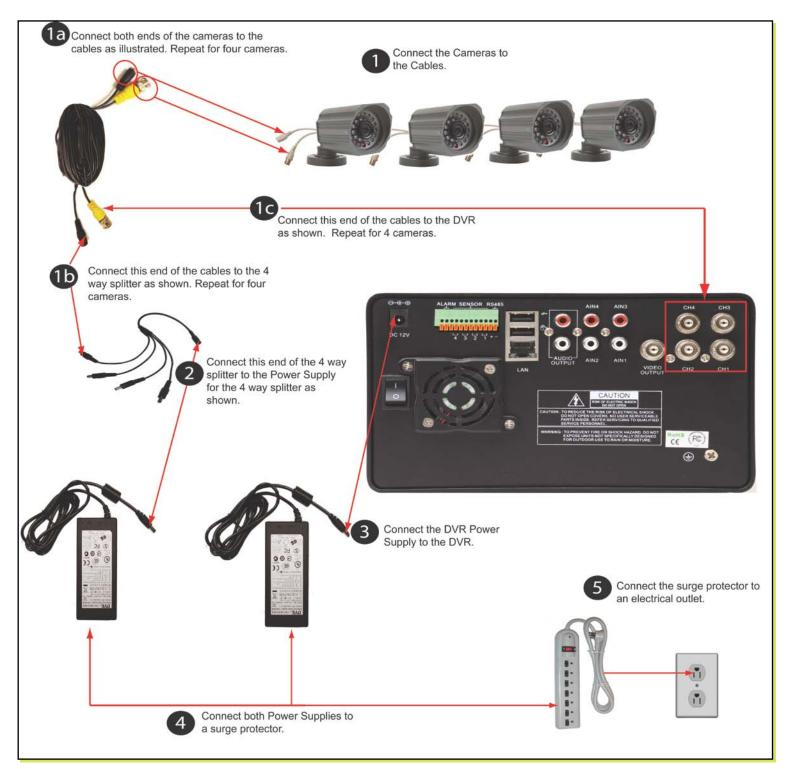
Please note that it is STRONGLY recommended to use a surge protector that is UL-1449 rated. Look for a clamping voltage of 330 or lower, a Joule rating of at least 400 and a response time of 10 nanoseconds or less.
